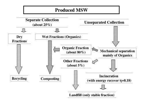
Figure 2. Sketch of the integrated waste management and treatment system considered as 2001 optimum scenario.
